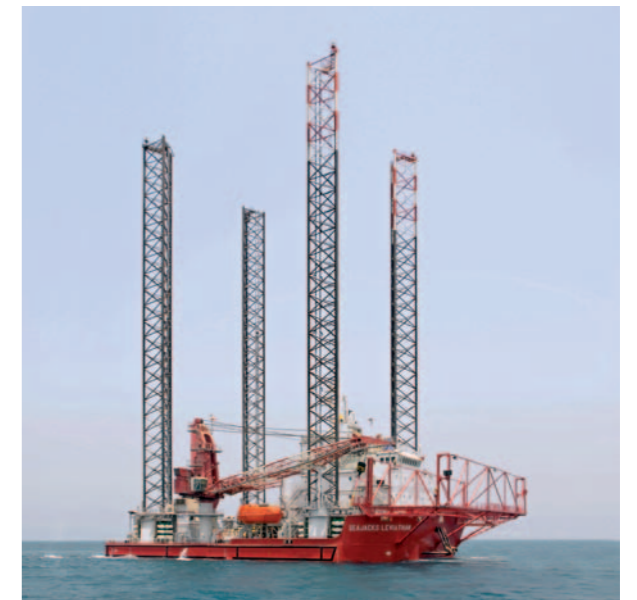
Wind turbine installation vessel Leviathan, which is to be used on Walney 2.
